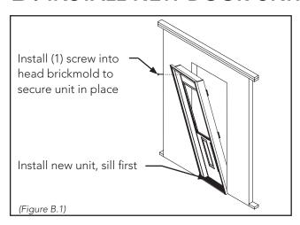
Wood shims can be placed between subfloor and sill to correct minor levelling and adjustments
