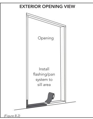
Opening preparation for replacement applications, remove existing door slab and jamb to expose rough opening.
