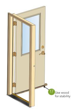
Step **17** Turn door upwards and place back onto wood support block from Step 1.
