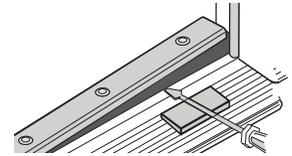
Loosen adjustment screws from underside of cap
