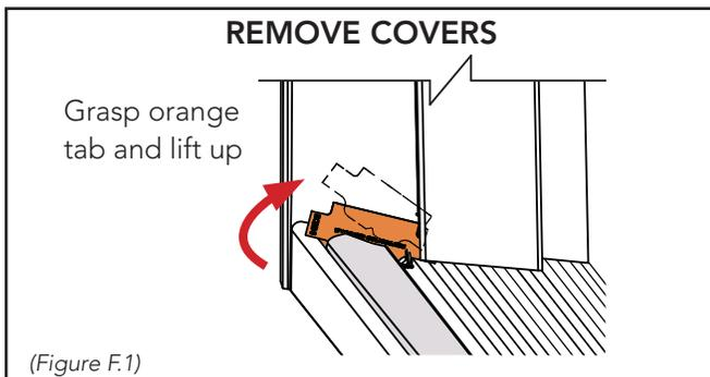
1 Remove the orange protective covers located at each jamb. Grasp tab on the orange protective cover, marked 'Pull-Up'. Gently and slowly, lift up and away from the sill base (pliers may be required). **DO NOT** remove any portion of foam gasket during removal of the orange tab. Note, a small portion of the outside gasket edge will be removed with protective cover, this is typical. (Figure F.1)
