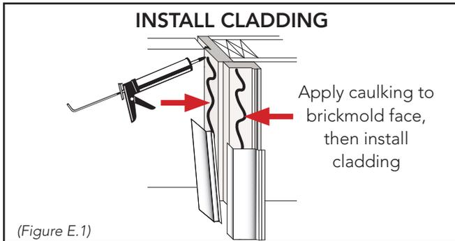
1 Apply a bead of caulking to the brickmold face in order to adhere cladding. Repeat for the jamb cladding if shipped loose. Then install all cladding. (Figure E.1)
