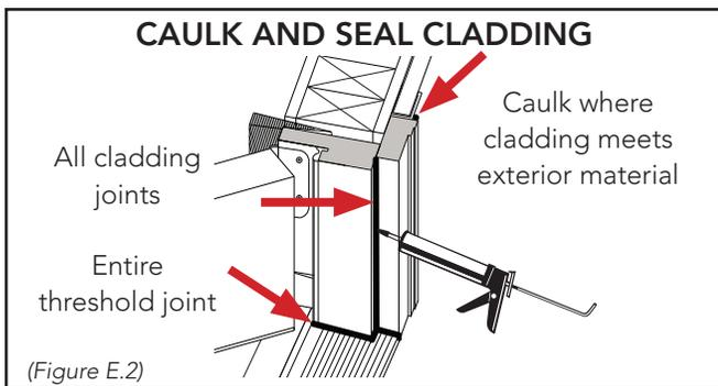
3 Caulk around ALL cladding joints. Be sure to apply caulking around perimeter where cladding meets exterior sheathing/material. (Figure E.2)
