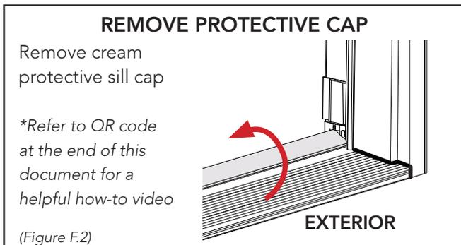
2 Remove the cream protective sill cap cover. For inswing door units, grasp cover from the exterior side, lift and roll toward the interior. The cap cover may break, this is typical. (Figure F.2)
