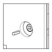
a. If the square spindles fell out of the lock when the escutcheons were removed, re-insert them into their hubs within the lock.
