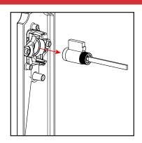
b. Remove the key cylinder from the escutcheon.
