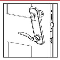
b. Carefully remove the plates from the door panel. **NOTE**: There are loose pieces that may fall out as the plates are removed - do not lose these pieces.
