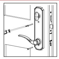
a. Remove the 2 mounting screws on the interior escutcheon that are securing both plates together. **NOTE**: Do not lose these screws. You will need them to reattach the handset.
