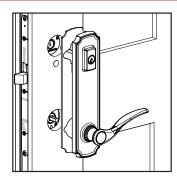
b. Start with the exterior escutcheon. c. With the interior escutcheon. If the gasket is still present, align it with inside face of the escutcheon. Guide the cylinder tailpiece and handle cartridge into the respective hubs on the lock hardware. Hold in place.
