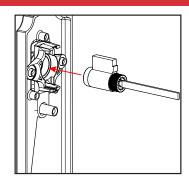
b. Insert the key cylinder into the upper hole from the back side of the escutcheon with the tab pointing up.
