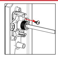
a. Remove the screw securing the current key cylinder. **NOTE**: Do not lose this screw. You will need it to install the new cylinder.
