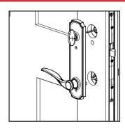
guide the thumb-turn receiving slot towards the cylinder tailpiece and align the handle cartridge with the spindle. Both escutcheons should lay flush against the door panel.
