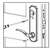
d. Secure the handsets with the mounting screws from the interior to exterior. Do not overtighten.
