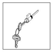
a. Remove the keys from the key cylinder.
