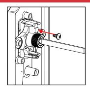
c. Secure the cylinder using the tapping screw you removed in step 2.
