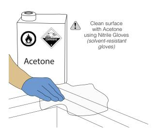
**Step 2 -** Using Nitrile gloves and a lint-free cloth dabbed with Acetone, gently wipe the frame to clean off any dust or residue from the surface.
