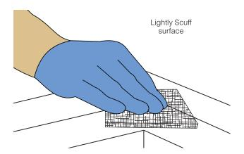
**Step 1 -** Using a Scotch Brite Pad or 320-400 grit sandpaper, lightly scuff sand the surface.
