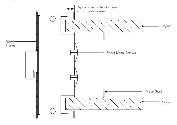
**Note:** Drywall must extend at least ½" into frame for Fire Rated Installation.
