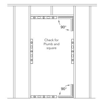
**Step 2**-Check frame opening for plumb and square.
