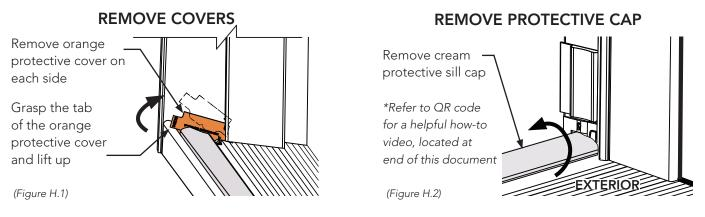
Remove the orange protective covers located at each jamb. Grasp the tab of the orange protective cover, marked 'Pull-Up'. Lift up and away from the sill base (pliers may be required). (Figure H.2)
