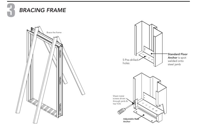
**Step 1**- With the frame plumb and the wood spreader in place, fasten frame sides to floor through the **Standard Floor Anchors** (see illustration) using the predrilled holes.
