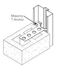
**Step 1**- Install Masonry T Anchors at hinge levels as wall is laid up. Use 3 anchors per side, 6 total for heights up to 7'-2". Add one more anchor per frame side for each additional 2 feet of height.
