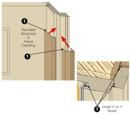
**Step 1-** Re-install brickmold and frame cladding and tack in place with 3/4" or 1" brads (see illustration).
