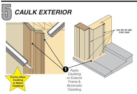
Step 1 - Using a ProVia color matched caulking or any other high quality caulking in accordance with ASTM C 920 Class 25, caulk the exterior frame and brickmold cladding (see illustration).
