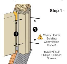
Secure the brickmold and jamb frame using #8 x 3" Phillips Flathead Screws as specified in the installation instructions by the Florida Building Commission.
