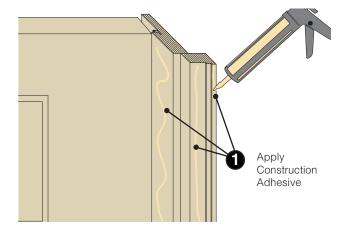
Step 1- Using a construction adhesive, apply ample beads of adhesive on both the frame and exterior of brickmold.
