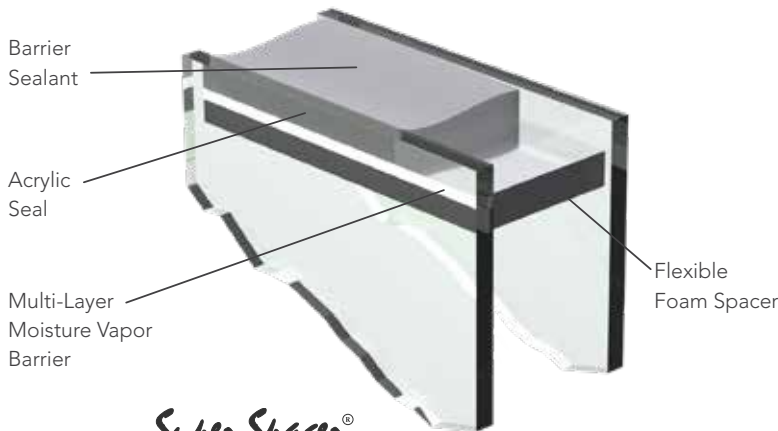
Super Spacer® Reverse dual seal technology
