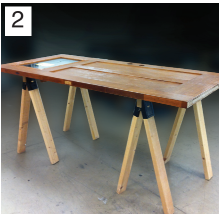
Step 2 Lay slab horizontal on sawhorses.
