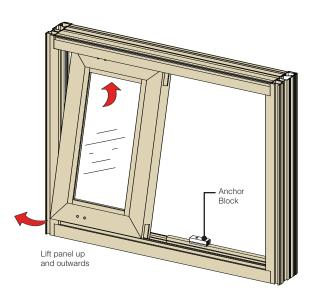
**Step 3-** Lift fixed sash up and tilt bottom outwards towards inside of home.
