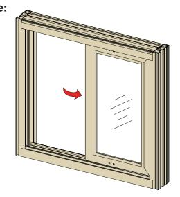
Step 2- Slide fixed sash towards fixed panel jamb and over anchor block.
