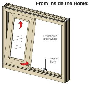
**Step 1-** Lift fixed sash up and tilt bottom inwards from inside of home.
