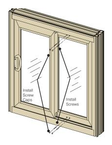
Step 3- Re-install screw cap covers on top and bottom rails of fixed sash.
